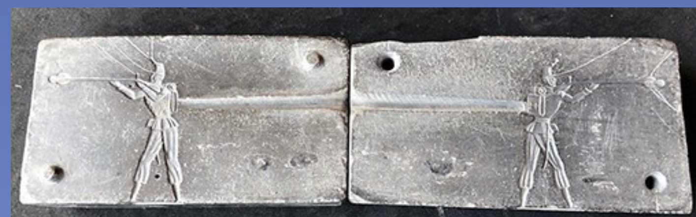
Figure 3. Example of a mold for a two-dimensional toy soldier, engraved in a block of slate, mid to late 19th century. Note the large channel for pouring in the molten metal and the smaller grooves to allow air to escape during the casting process. https://www.aebn.com/item/A-Fine-Engraved-Mid-Late-19th-Century-Flat-Tin-Soldier-Slate-Mold-33256643549
